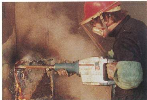
Withstands the formidable core drill and heavy tool attack UL TL 15.
