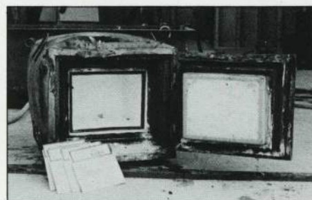
The MVP-101 after testing — While the outside is charred and swollen from heat, both the media storage area and data contained on the diskettes remained intact.
