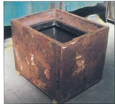
One Piece Composite Body Casting
