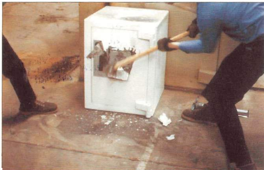
Typical Underwriters Lab. Tool Attack
